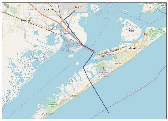
The High Island Pipeline System gathers crude oil from offshore facilities and transports the crude to a facility in Texas City. The onshore portion makes landfall near Eight Mile Rd., crosses Galveston Bay and terminates at the Texas City Facility on Loop 197 South.
